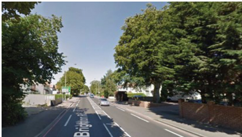
Removing centerlines from this and other British streets reduced driving speeds an average of 7 mph. (Source: Google Streetview)
