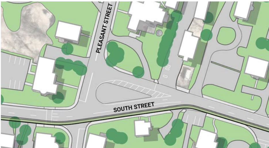
Excess pavement at an important intersection.
