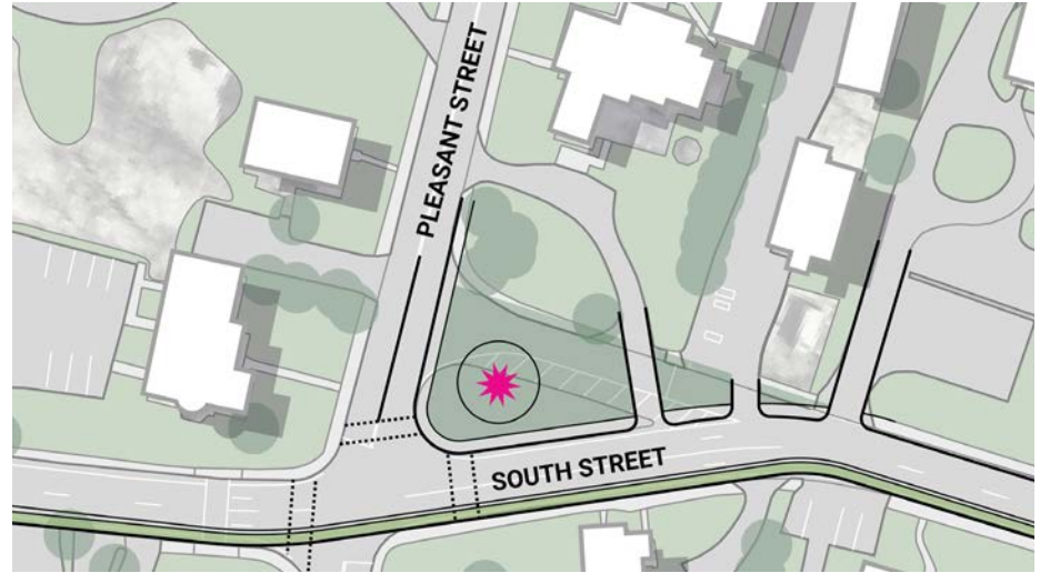
Removal of the unnecessary slip lane creates an expanded green.
